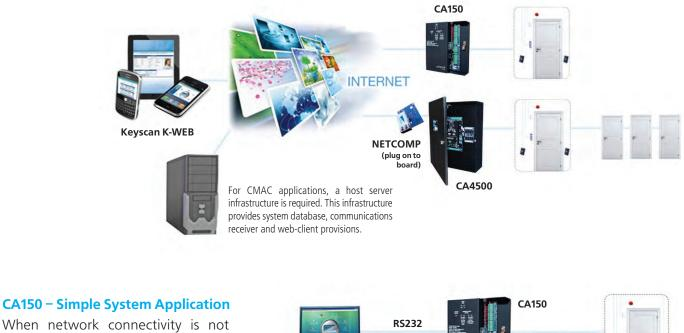
When network connectivity is not available, the RS232 communication port provides a convenient way to configure and download events to the CA150 when needed.
